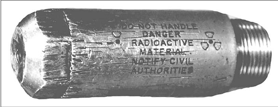
Figure 10: Example of a Radioactive Sealed Source That Contains Americium-241
