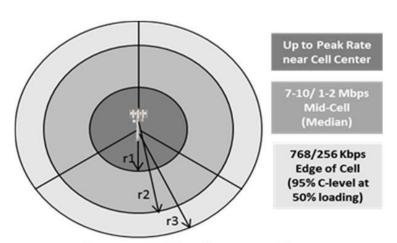
Notes: Cell coverage radii (r1-r3) per sector will vary depending on transmit power, antenna gains, antenna heights, and the coverage topology (urban, suburban, rural). Data speeds will vary based on number of simultaneous users, and the priority of the users, with public safety having higher priority to ensure these optimal data speeds and latencies are provided.
